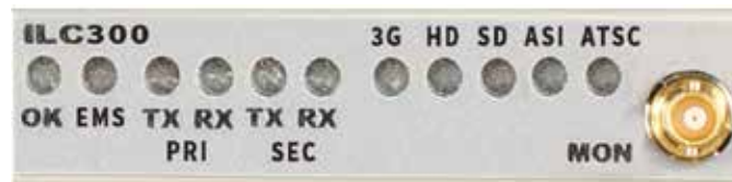
Figure 7. ILC300 Front Panel Status LEDs and Monitor Connector
