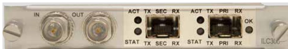
Figure 8. ILC300 Rear Panel Status LEDs
